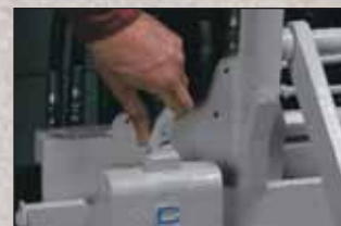
Platens are hung like conventional forks so spacing can be adjusted in seconds (carriage mount modes).
